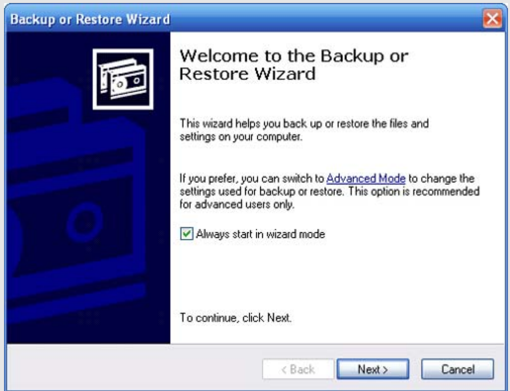
Figure B: The Windows Backup Or Restore Wizard simplifies backup creation and helps ensure that you don't miss critical configuration settings (such as scheduling the backup to occur daily or configuring an Incremental versus a Normal backup).
