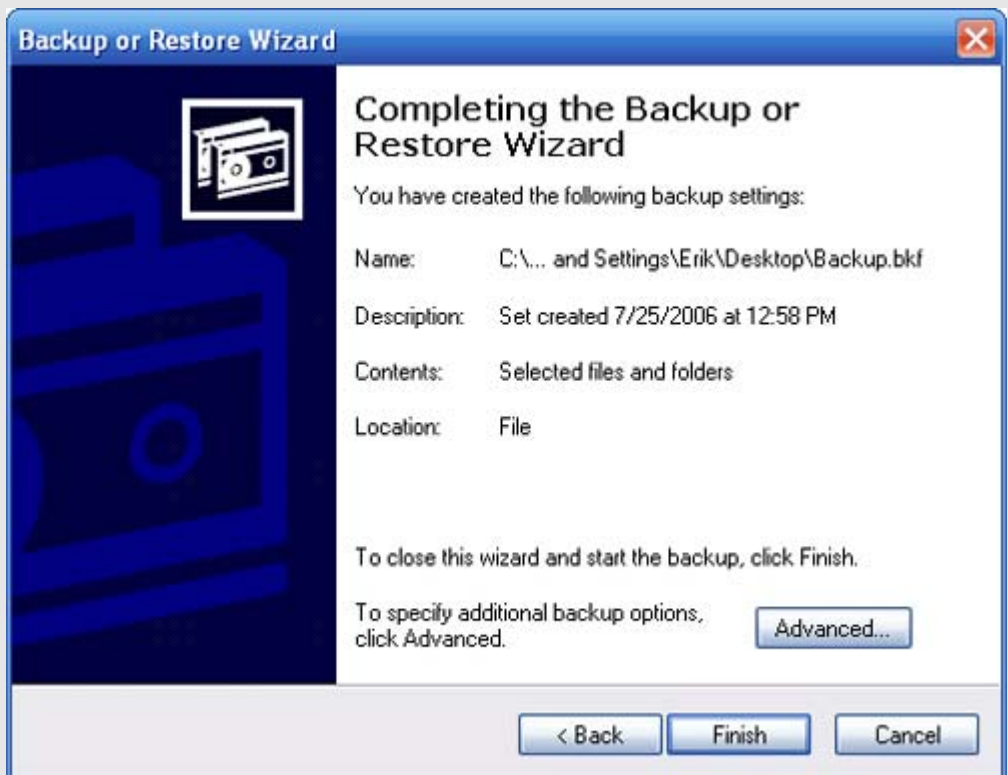
Figure C: The wizard's summary screen leads you to believe you're just about finished configuring the new backup; you're not. You still need to configure advanced settings.
